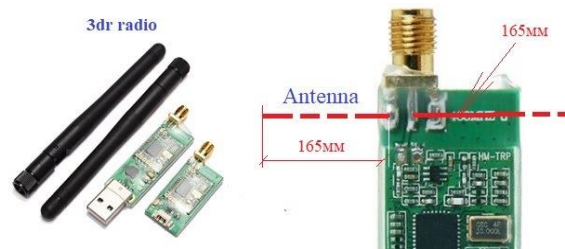
Figure 14 The modified antenna-dipole 3DR modules with the frequency of 433 MHz.
