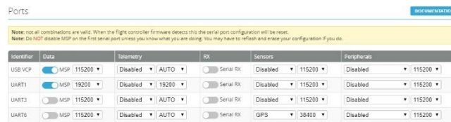
Figure 6 The installing ports for an airplane with telemetry.
